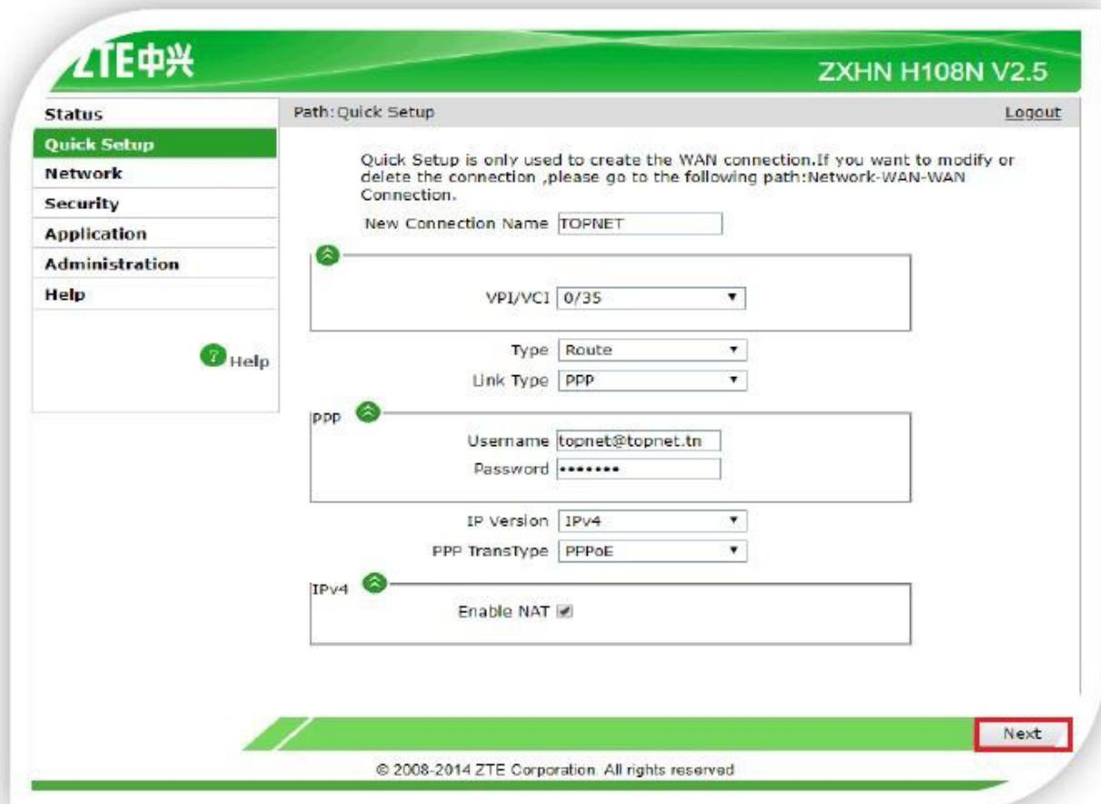
The screenshot shows the ZTE ZXHN H108N V2.5 web interface. The top navigation bar includes the ZTE logo, the model name 'ZXHN H108N V2.5', and a 'Logout' link. The left sidebar menu has links for 'Status', 'Quick Setup' (which is highlighted in green), 'Network', 'Security', 'Application', 'Administration', and 'Help'. The main content area is titled 'Path: Quick Setup' and contains the following configuration fields:
